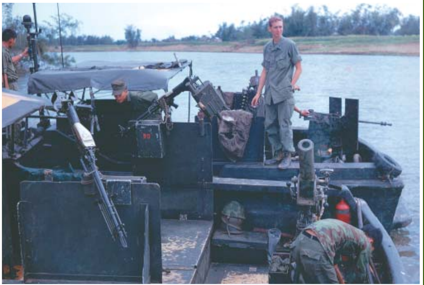
Above: Two Patrol Boat Rivers await a CDT3 crew for riverine Ops near the DMZ. Note early model 40mm grenade launchers, flex mounted M-60s and M-2s and 81mm mortar. Below: A US Navy EOD Petty Officer directs the laying of the Mark 8 hose charges on the Song Hau Giang.
